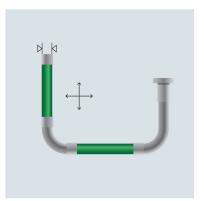
Use a "U" shaped assembly in order to absorb movements or vibrations.
