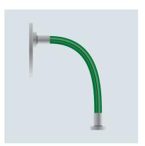
Do not allow twisting movements, but move in the required direction without wringing.
