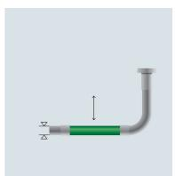
Do not allow a single hose to absorb movements with different directions; use instead the line of the angle.
