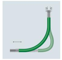
Assemble horizontally with respect to the direction of the movement.
