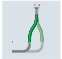
The fittings should be weld after the assembly only when there is no other choice. In such case, make sure that the hoses are made with high-temperature resistant materials. Do not overheat too much the coupling, but cool down and keep away from the burner.
