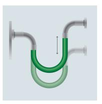
Do not allow axial movements; assemble perpendicularly to the axis of the hose.
